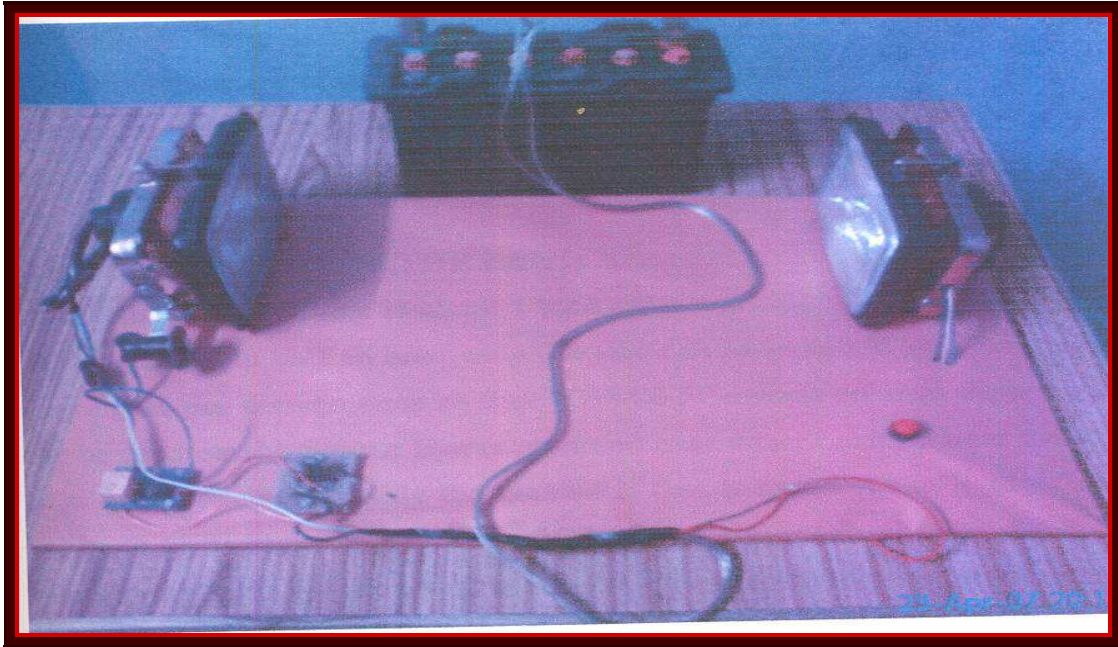
Fig.3 Experimental setup for electronic headlamp glare management device.
